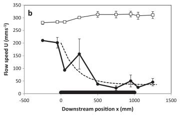
**Fig. 3.** Downstream development of the mean flow speeds over the canopy  $(U_a)$ ; clear symbols) and within the canopy  $(U_b)$ ; filled symbols) for (**a**) short-leaved and (**b**) long-leaved seagrass canopies. The dotted line indicates the predictions of the model of Chen et al. (2013)—see text for details. The thick black lines indicate the location of the seagrass canopy.
