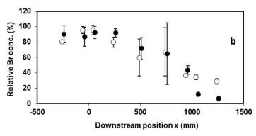
**Fig. 4.** Relative bromide concentration, as defined in equation (1), in the pore water measured after 24 h of running the flow, for (a) the short-leaved seagrass canopy; and (b) the long-leaved seagrass canopy. Clear symbols represent relative bromide concentration in 0.01 m depth; filled symbols represent relative bromide concentration in 0.02 m. Error bars show standard deviation of samples measured at the three parallel locations for each *x*-position shown in Fig. 1b.
