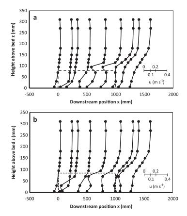
**Fig. 2.** Flow profiles for **(a)** short-leaved and **(b)** long-leaved seagrass canopies. Filled symbols represent u profiles (normalized to u at z = 0.3 m). The dotted lines indicate the location of the canopy where long-leaved seagrass bent to similar height as short-leaved seagrass height. The velocity magnitudes are indicated by the scale bars.
