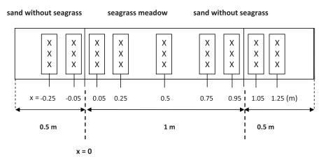
**Fig. 1.** (a) Plan view of the racetrack flume tank at NIOZ, Yerseke; (b) Plan view of the simulated seagrass meadow placed in the test section of the flume, showing locations of measurements of nutrient penetration. [Color figure can be viewed in the online issue, which is available at wileyonlinelibrary.com.]
