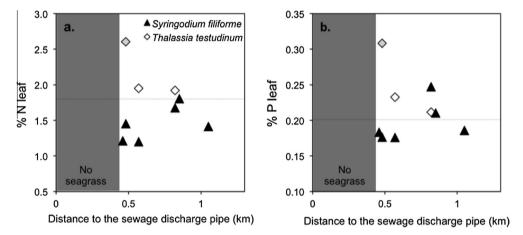
Fig. 2. Distance analysis on the effects of a emergency overflow discharge pipe on (a) leaf % N and (b) leaf % P concentrations of *Thalassia testudinum* and *Syringodium filiforme* in Piscadera Bay. Dotted lines indicate the limitation levels (1.8% N and 0.2% P) for seagrasses, as stated by Duarte (1990). Displayed values are means and error bars present standard errors.
